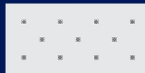
**11 per 4' x 8' board achieves FM 1-90** with adhered non-reinforced-membrane applications over a minimum 22-gauge steel deck or structural concrete deck.
